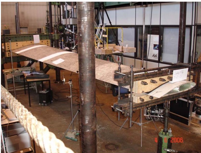
Figure 5.1.7 - Flapwise bending
