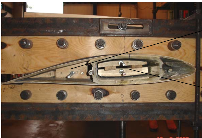
Figure 5.1.6 – Stiffening of load clamp (clamp 3)
