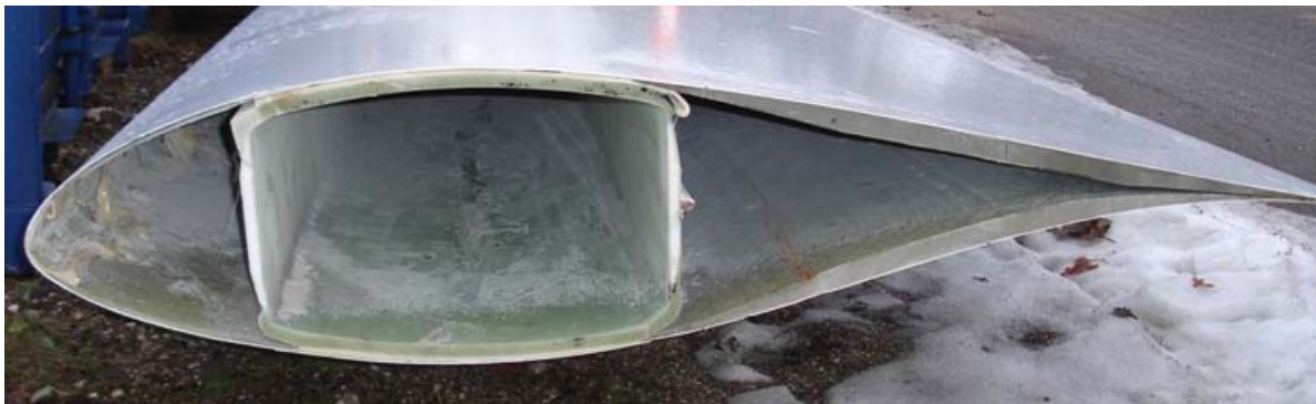
Figure 6.2.13 - Cross section picture of the real blade at R10.7
