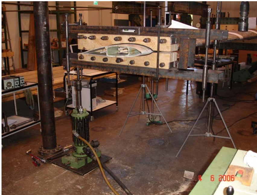
Figure 5.1.9 - Flapwise bending and torsion
