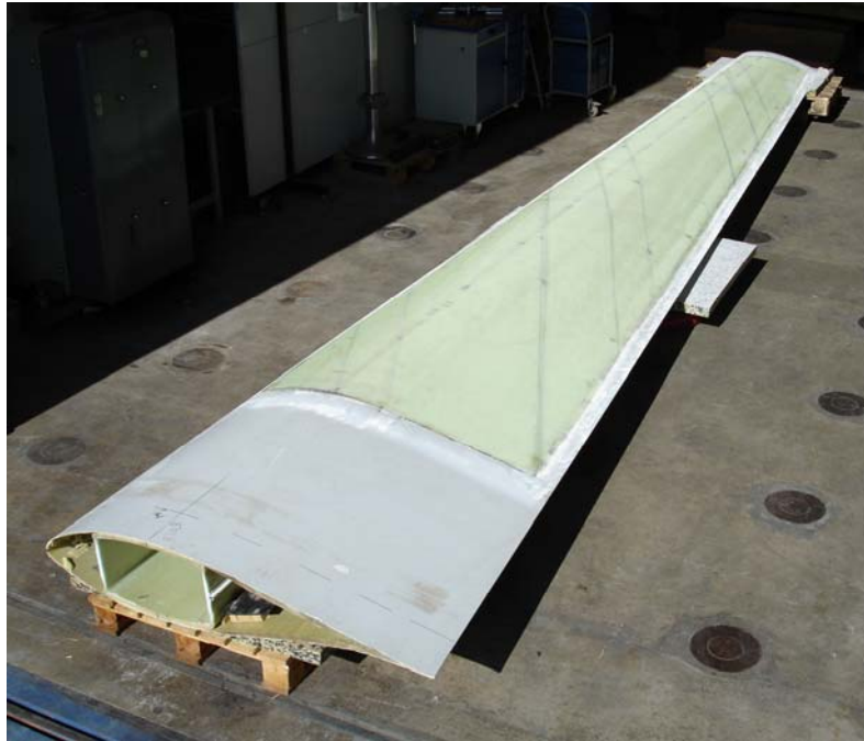
Figure 5.6.2 – Extra UD lamination
